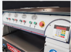
Operator controls with digital thickness control unit
