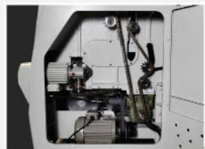
Powerful chain driven upper and lower rollers and variable speed feed motor
