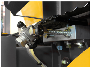
Blade spray mist lubrication system
