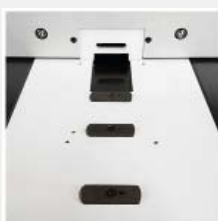
Simple drawer location stops and left and right limit switches for drill location
