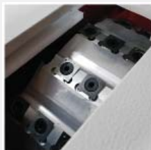
Insert cutterhead remains below the table under a guard until in operation
