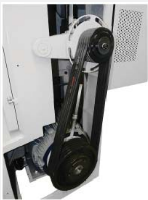
Powerful 50 HP motor with 5 v-belt drive
